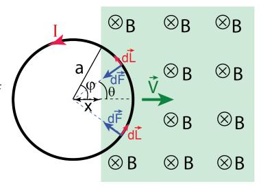
increase by  $d\Phi = BdA$  where dA is the area of the strip of the height  $2\sqrt{a^2 - x^2}$  and width Vdt:
